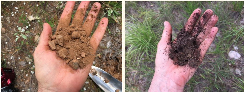
After a squeeze, degraded (left) fall apart because they lack SOM, while healthy soils (right) retain a loose ball.
